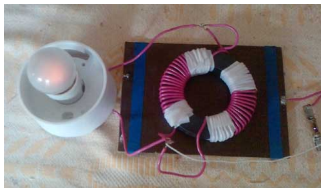
Fig. 8 Observation of the electro-radiant effect according to the diagram in Fig. 6 with a different configuration of the capacitor electrodes.
